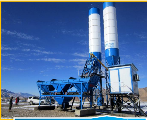
Concrete mixing plant-35m 3 / hour
